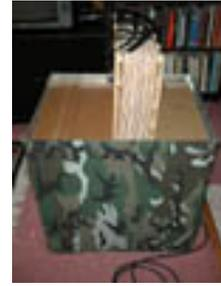
A standard plant press will sit on the lower angle of the zinc at the top of the dryer. Close off any space on either side of a thin plant press by using a board or cardboard. Tighten and flip the press daily or as needed. Drying time varies according to several factors including specimen characteristics, humidity, and air circulation. Recheck specimens after they have been off of the dryer for a day or two to see if more drying is actually required.
