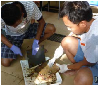
All sides of the plates are scraped into a clean photo tray
