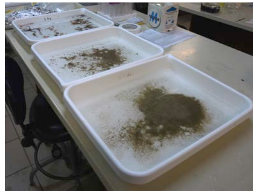
The three fractions collected with the 2-mm Sieve (left) 500- \mu m sieve (middle) and the 106- \mu m sieve (right)
