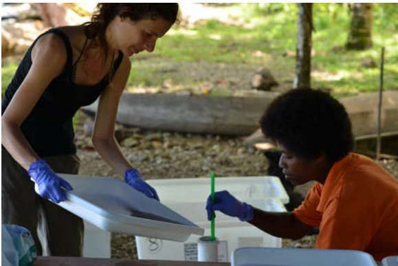
The 500- \mu m and 106- \mu m are concentrated on a 40- \mu m nytex mesh
