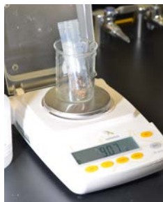
Step 7 to 11: Organic matter is weighed and half is grinded for DNA extraction.
