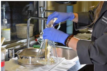
Steps 3 to 6: Organic matter is removed from original sample through decantation.
