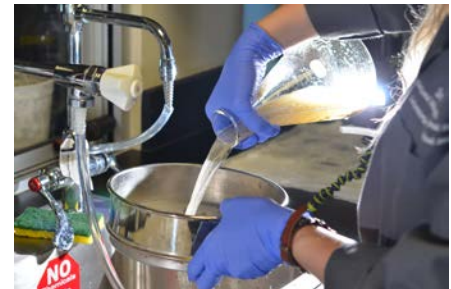
Steps 3 to 6: Organic matter is removed from original sample through decantation.
