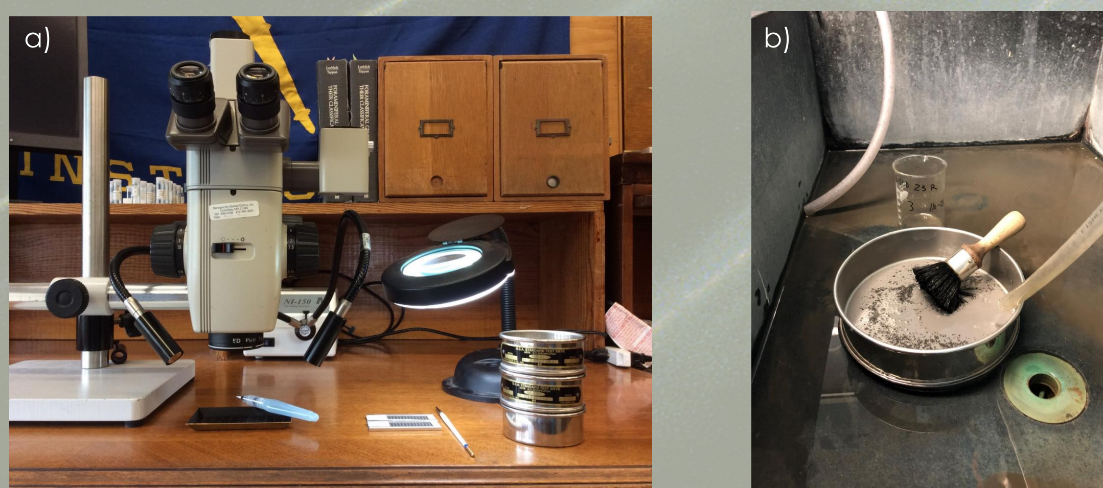
Figure 2: a) Nikon SMZ-U light microscope used for examination of foraminiferal assemblages. b) Wet-sieving process with >38 μm sieve. (photos: Becca Goughnour)
