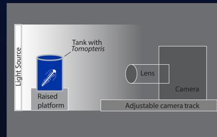
Fig 2. Setup for *Tomopteris* filming
