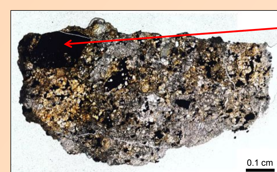
Melt shows up dark in plain and polarized light, but light gray under reflected light, distinguishing it from metal.
