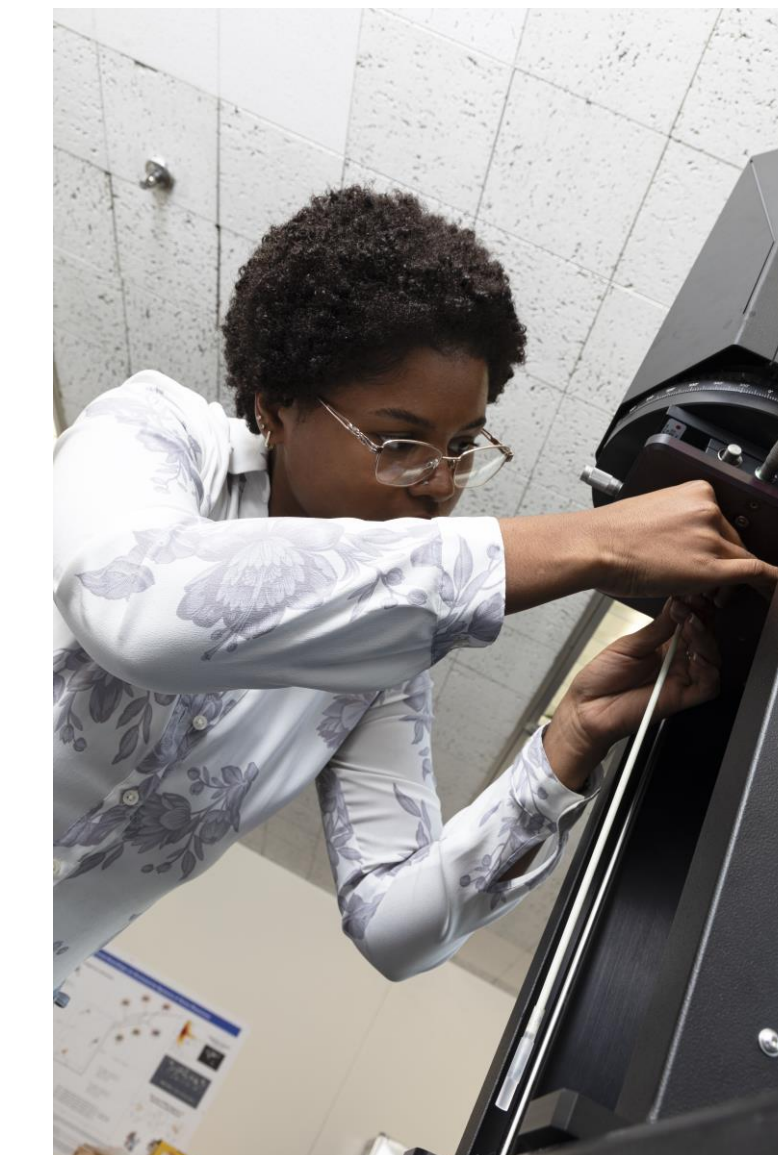
Fig 3: Ie'Jana Woodley attaching sample rod to VSM for magnetic measurements NMNH Photo, 2024
