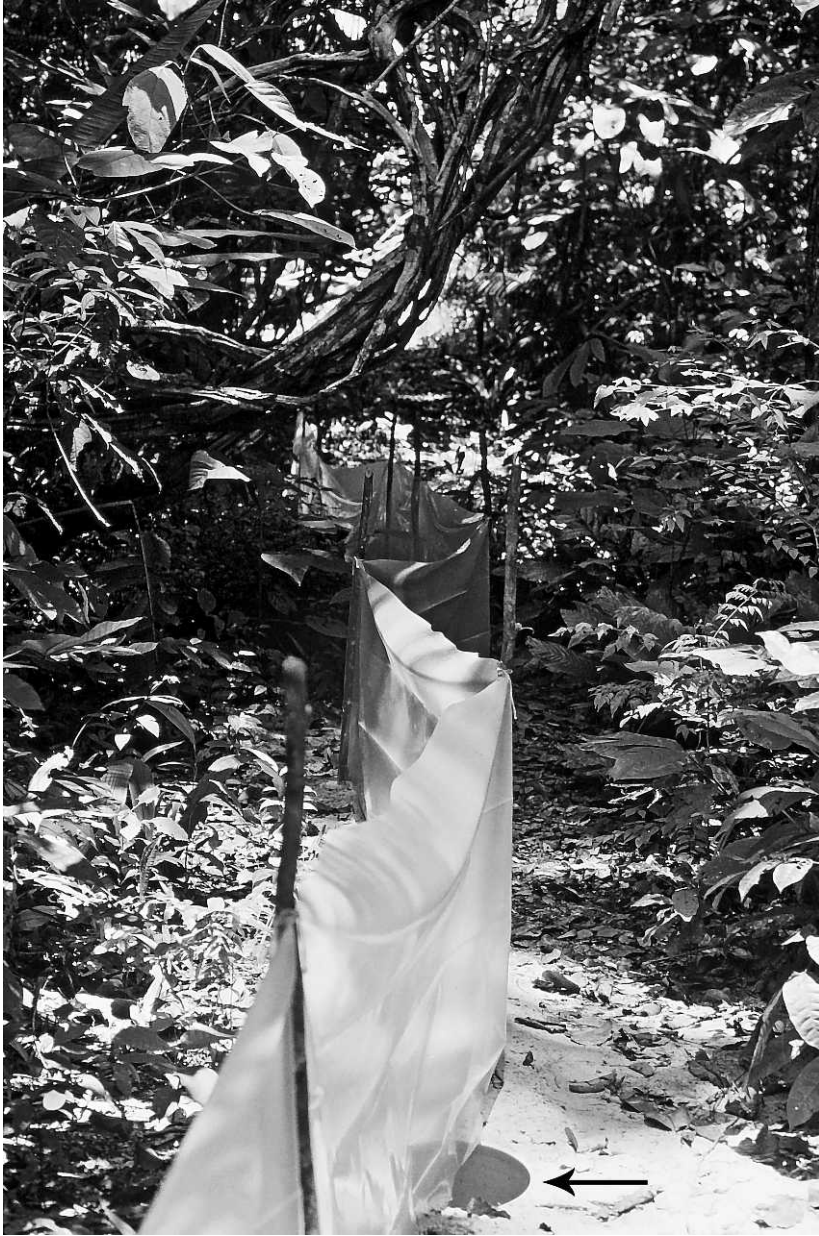
Fig. 1. Trapline of drift fence (plastic sheeting stapled to cut saplings hammered into ground) and pitfall trap (arrow; 20 liter plastic bucket buried with brim flush to ground). Plastic sheeting crosses the middle of the open top of the bucket to allow catching things from either side.
