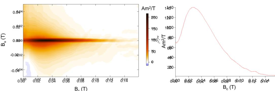
**Figure 4.** (Left) FORC diagram from sample HP31435 (95.81 m depth) indicated by the red arrow in Figure 3. (Right) Coercivity profile of HP31435 (95.81 m) across where B<sub>u</sub>=0.
